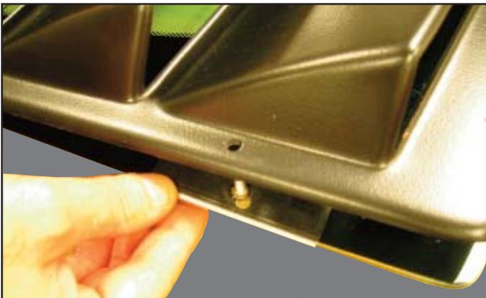
5. Lift up the sides of the louvers and insert the five (5) bent mounting brackets (1 per side & 3 along the top) making sure that the bent edges are facing outwards and the mounting studs are protruding through the existing holes in the louvers.
