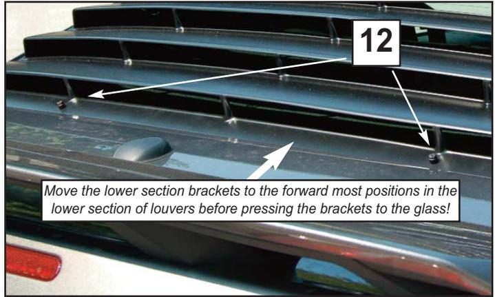
Move the lower section brackets to the forward most positions in the lower section of louvers before pressing the brackets to the glass!
