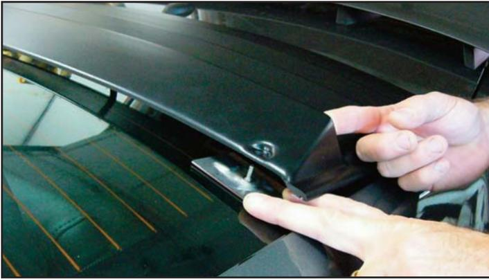
9. Place only the lower section of the louver on the rear glass over the previously installed lower brackets.
